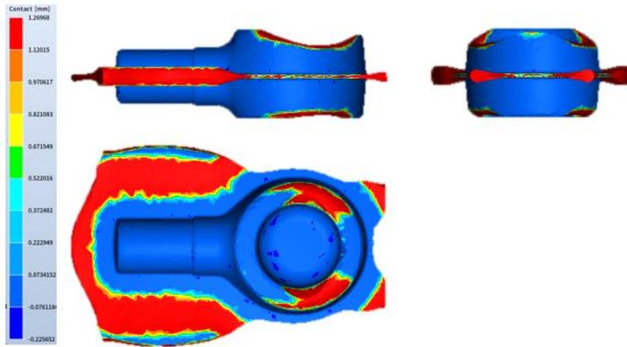
Figure 4: Filling state of the part after pre-forging and final forging process
