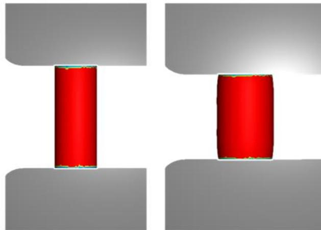
*Figure 5: Billet view before and after upsetting process*
