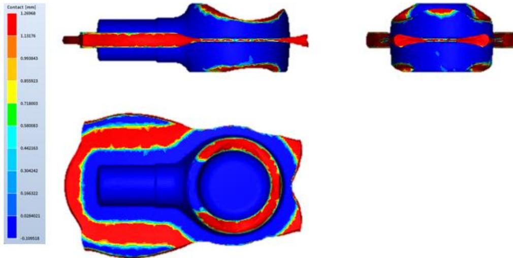
Figure 3: Filling state of the part only in case of final forging
