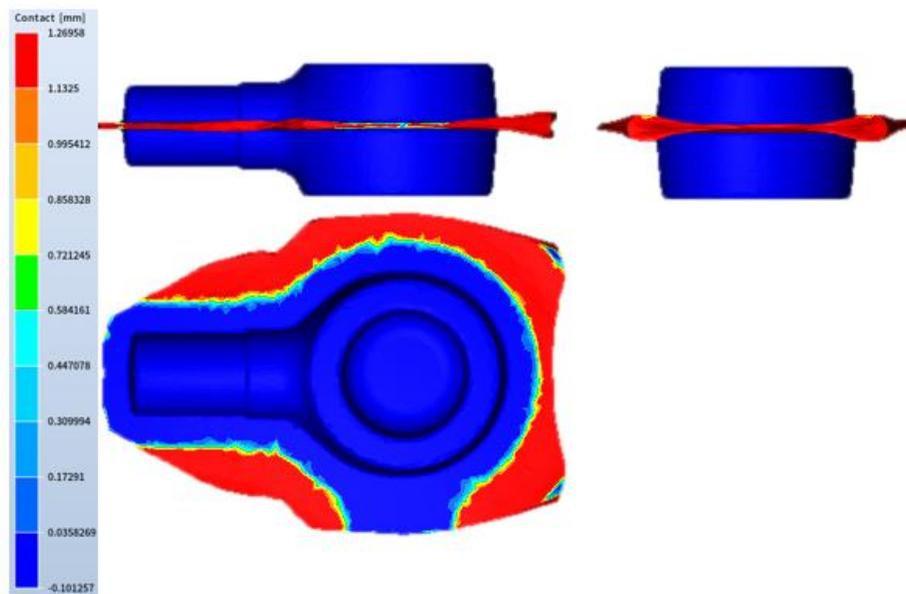
Figure 9: Filling state of the part after upsetting, shaft crushing, pre-forging and final forging process
