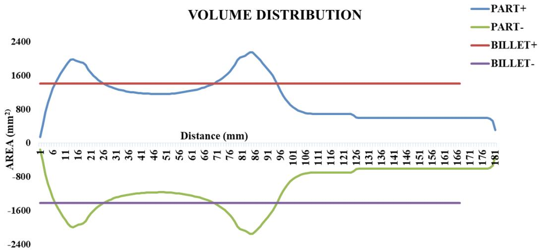
Figure 2: Volumetric distribution graph for determination of pre-forming
