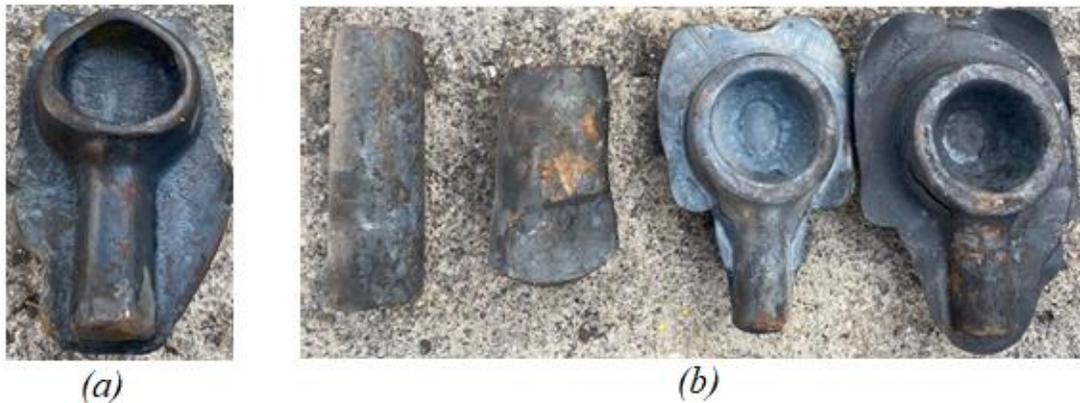
Figure 10: (a) Part forged without pre-forming (b) Pre-formed and final view of part
