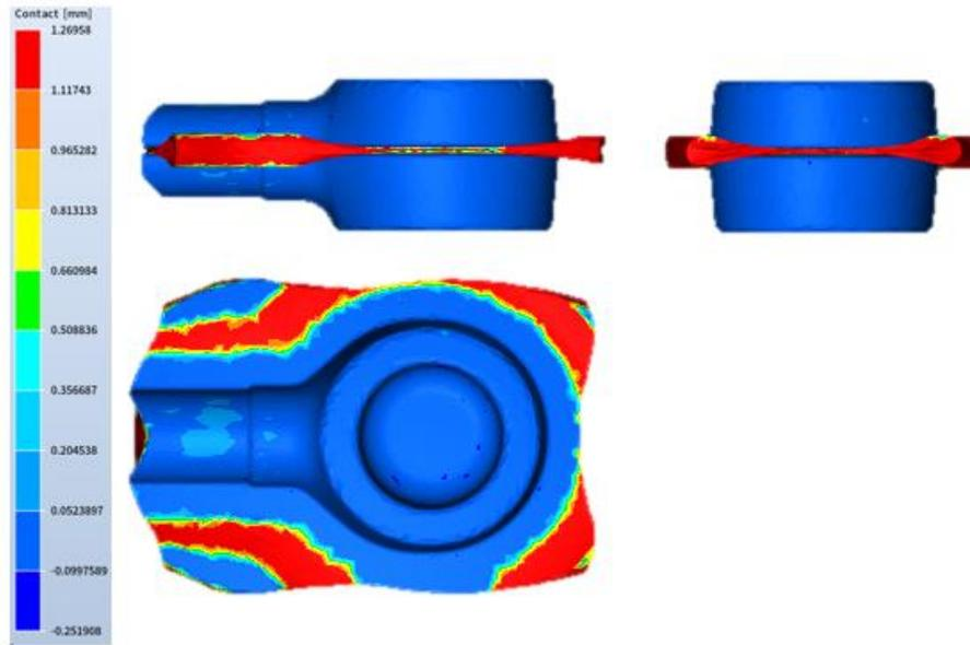
Figure 6: Filling state of the part after upsetting, pre-forging and final forging process
