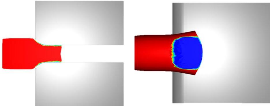
Figure 8: Billet view after shaft crushing process
