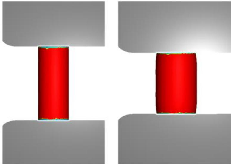
Figure 7: Billet view before and after upsetting process
