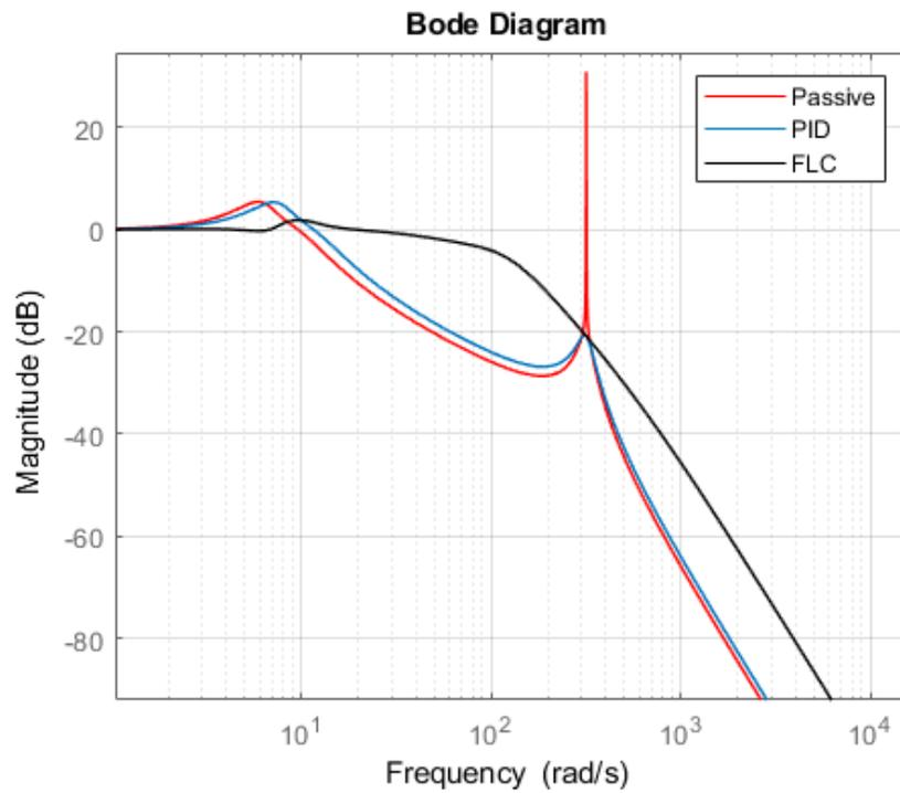
Figure 10: System Frequency Response
