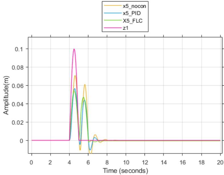
Figure 8: System Response for Second Disturbance
