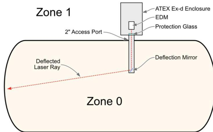
Figure 1: Schematic overview of the compact non-intrusive measurement system.
