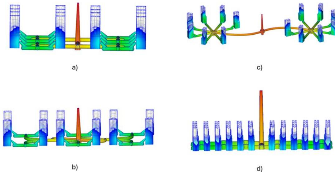
Figure 4: Filling behavior at 75% of the injection stage for the four runner designs.
