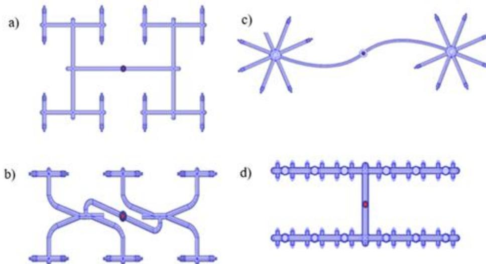
Figure 3: Mold layout and cavity arrangement for multi-cavity runner evaluation.
