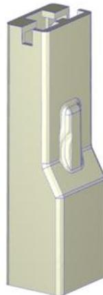
Figure 2: 3D model of the insulator used in the study.
