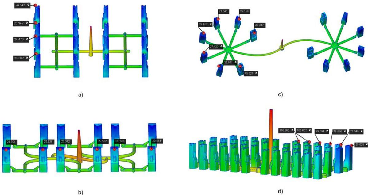
Figure 6: Filling behavior at 100% of the injection stage for the four runner designs.
