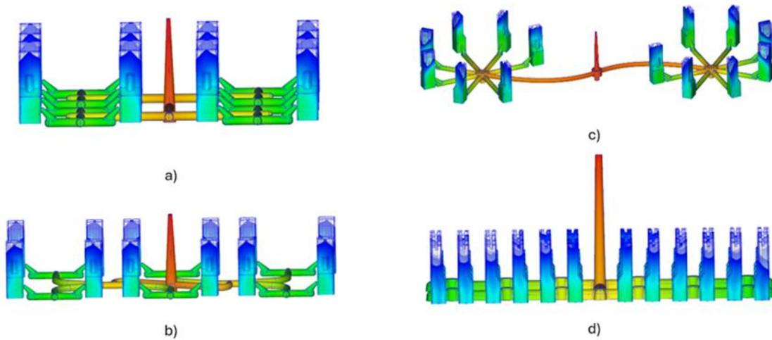
Figure 5: Filling behavior at 90% of the injection stage for the four runner designs.
