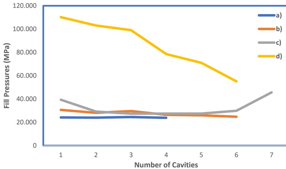
Figure 7: Fill-end pressure distribution for the four runner designs.
