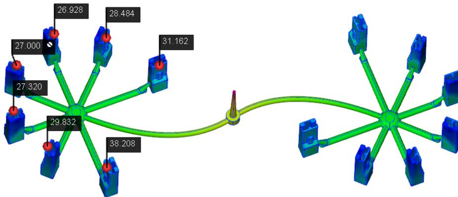
Figure 8: Star-type Runner Extended by 20 mm and Measured Pressures at Probes.
