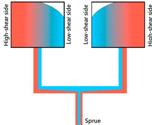
Figure 1: Effect of low shear rate and high shear rate within the runner.
