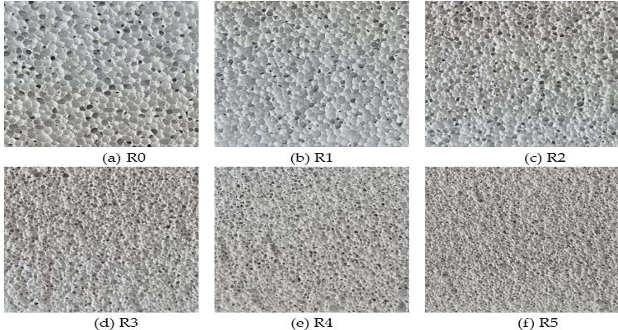
Figure 2: Images of AAC thermal insulation board with varying admixture of R, acquired along the expansion direction and cropped to 490 x 490 pixels: (a) 0%, (b) 0.1%, (c) 0.25%, (d) 0.50%, (e) 0.75%, (f) 1%
