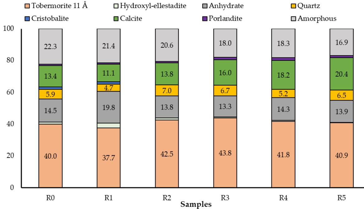
Figure 7: QXRD analysis of samples with varying R dosage (wt. %)
