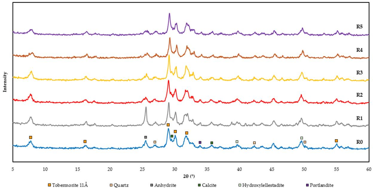
Figure 6: XRD patterns of AAC thermal insulation board specimens with varying R contents
