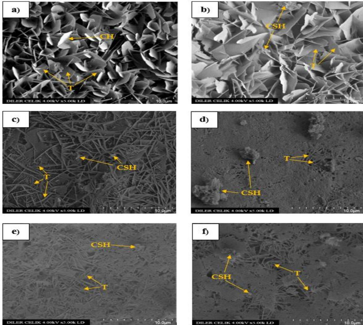
Figure 8: SEM images of AAC thermal insulation board samples containing R in various proportions at 5000x magnification (a) R0, (b) R1, (c) R2, (d) R3, (e) R4, (f) R5 (CH: portlandite, CSH: Calcium-silicate-hydrate, T: Tobermorite)
