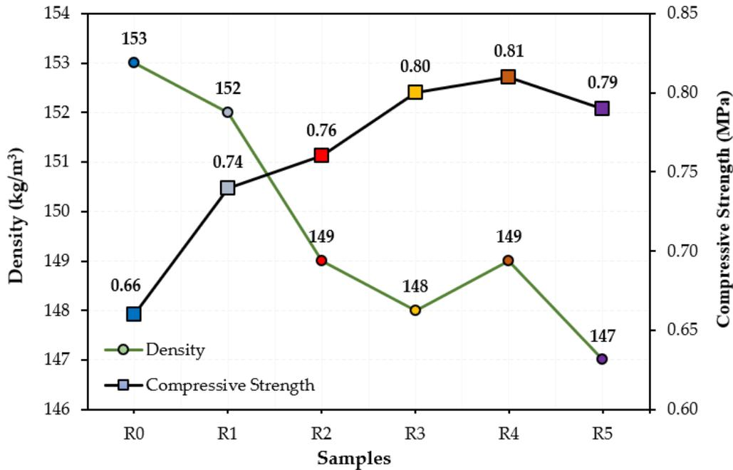
Figure 4: Effect of adding R to AAC thermal insulation board on density and compressive strength
