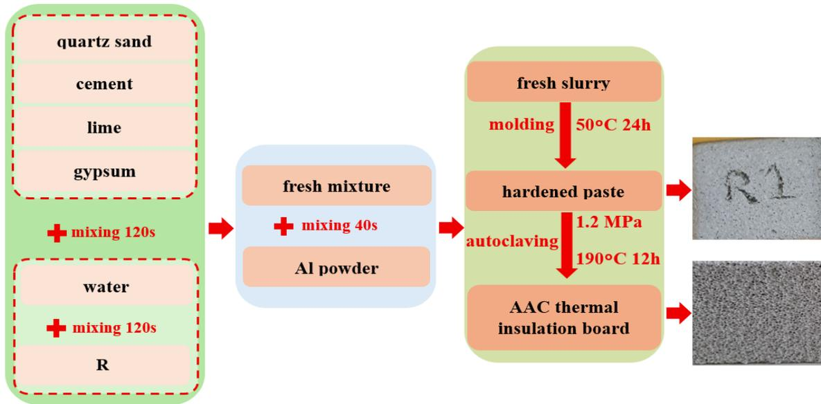
Figure 1: Preparation flow chart of AAC insulation board samples incorporated with R
