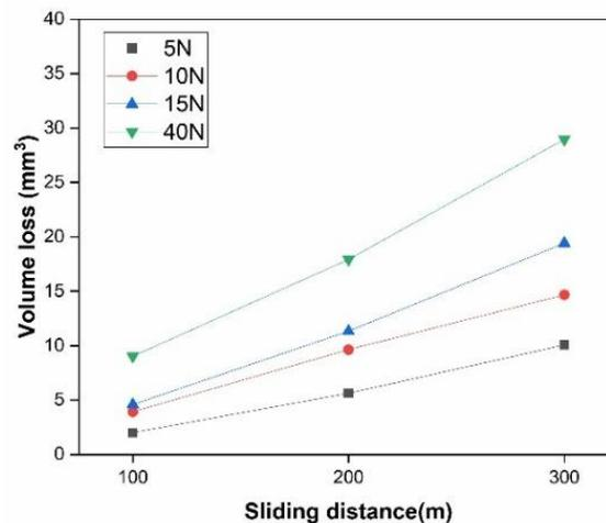
Figure 7: Volume Loss Depending on the Sliding Distance Under 3 m/s Sliding Velocity
