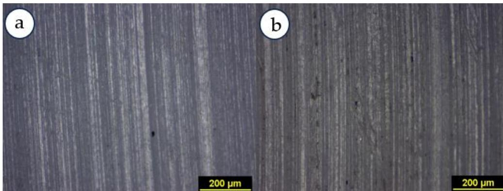
Figure 11: Surface Wear Traces at Sliding Speeds of a. 3 m/s and b. 4.5 m/s
