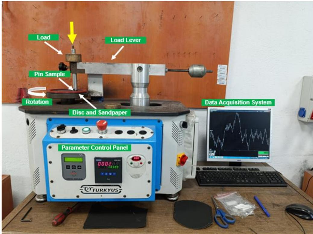
Figure 5: Pin-on Disc Wear Tester
