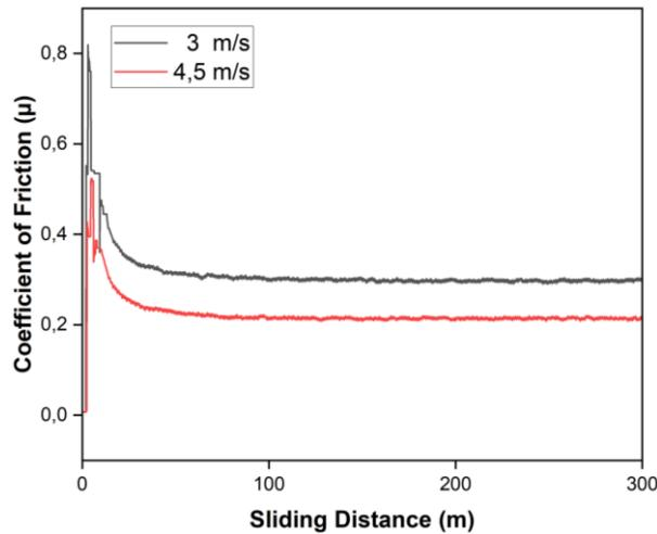
Figure 9: The Coefficient of Friction Depending on the Sliding Distance Under Sliding Speeds of 3 m/s and 4.5 m/s
