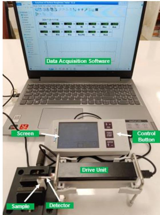
Figure 6: Surface Roughness Measurement Device
