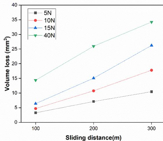
Figure 8: Volume Loss Depending on the Sliding Distance Under 4.5 m/s Sliding Velocity
