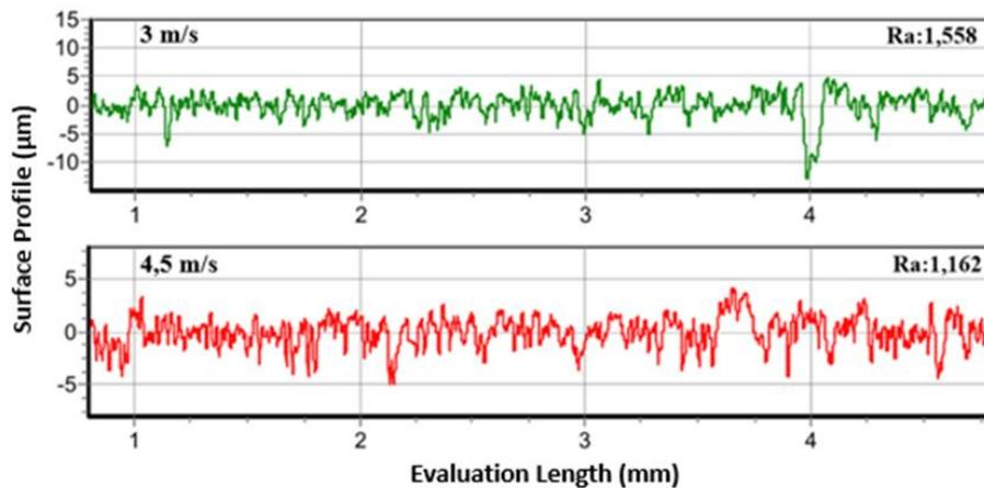
Figure 10: Surface Roughness Measurement Results at 3 m/s and 4.5 m/s Sliding Speeds
