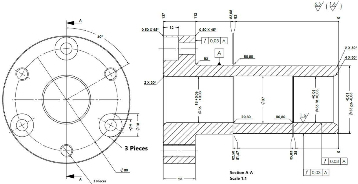
Figure 1: The Bushing Technical Drawing
