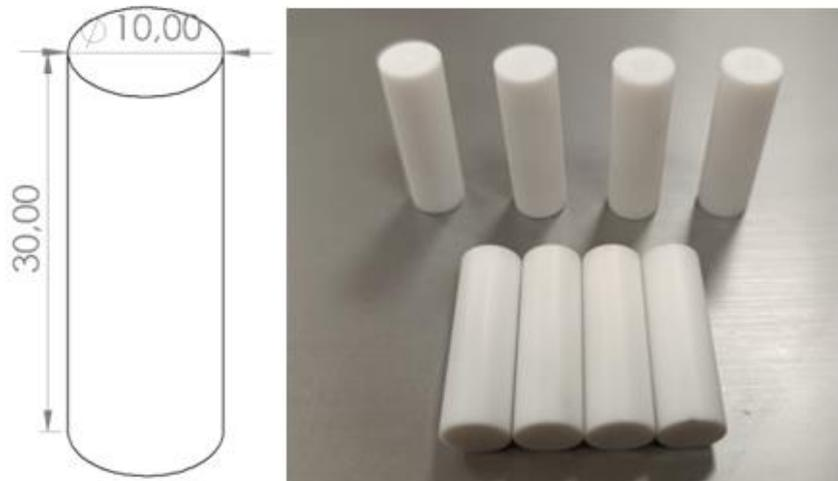
Figure 3: Wear Test Sample Dimensions and Sample Images
