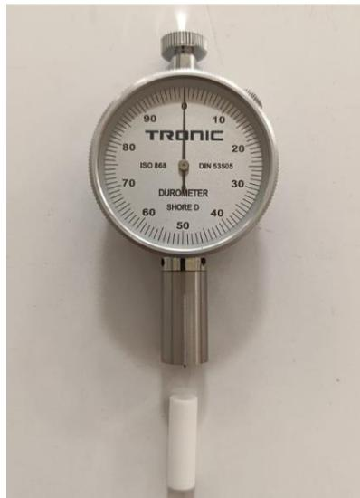
Figure 4: Hardness Measurement with Durometer
