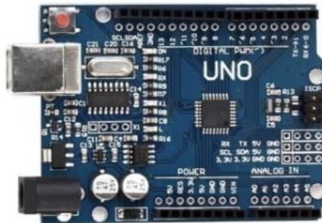
*Figure 2: Arduino UNO Card*
