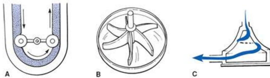
Figure 1: A. Roller Pump, B. Impeller pump, C. Centrifugal pump
