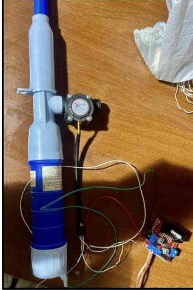
*Figure 6. Connection of the Water Flow Sensor and Motor Driver to the Pump*
