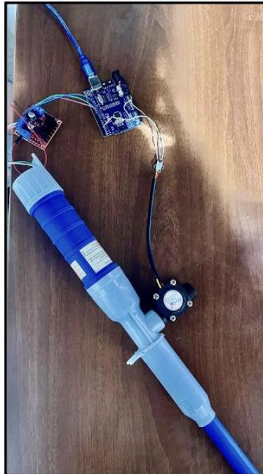
*Figure 7. Connection of Arduino UNO Board*
