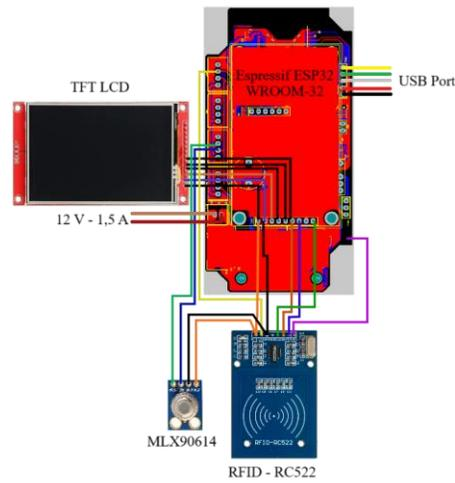
Figure 2: Hardware Circuit Diagram
