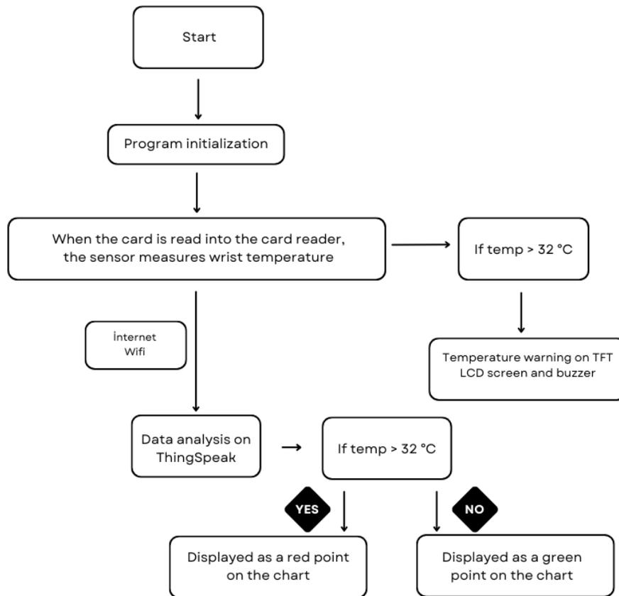
Figure 3: Flowchart Related to the Operation of the Hardware
