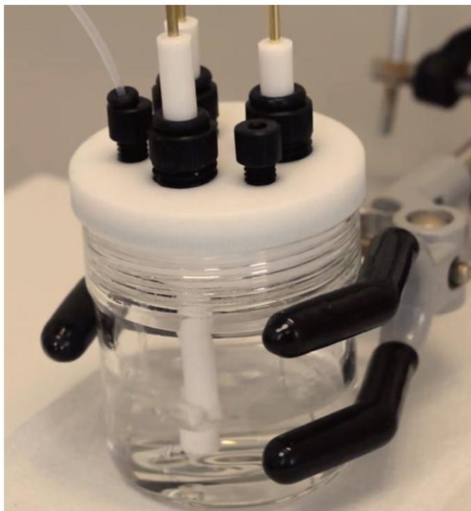
Figure 1: Electrochemical cell and triple electrode system
