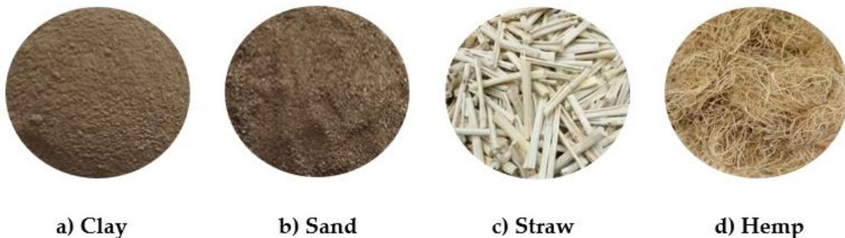
*Figure 4: Eco-friendly building materials: clay, sand, straw and hemp.*
