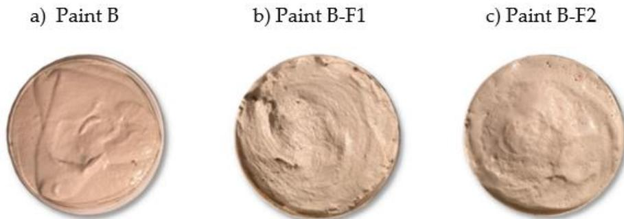
Figure 6: Visual comparison of paint B before and after the addition of fillers.
