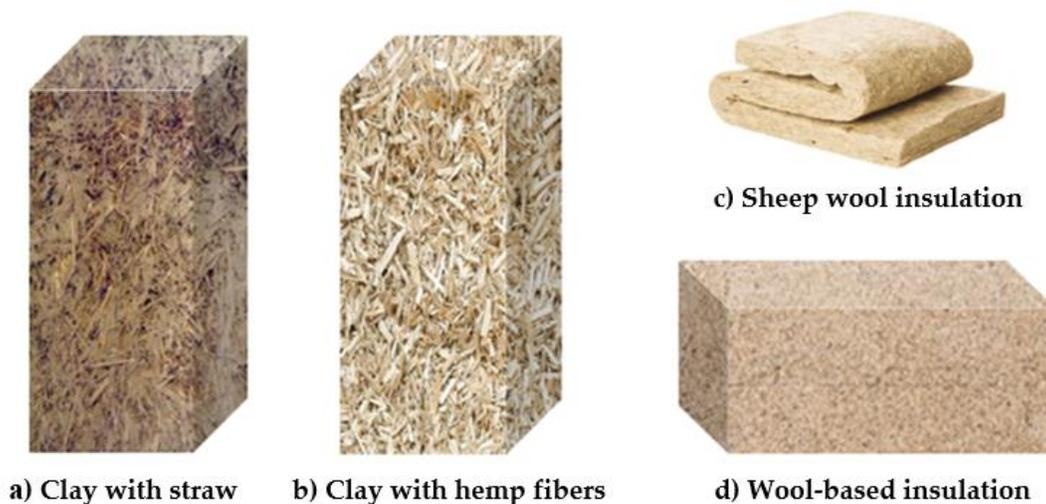
Figure 5: Natural insulation materials and raw components for earthen plasters.
