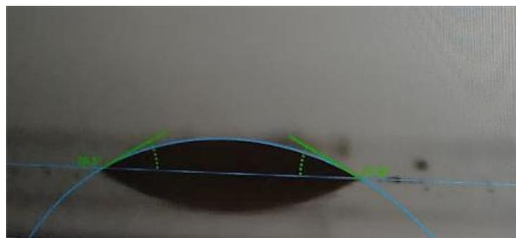
Figure 1: Contact angle measurement
