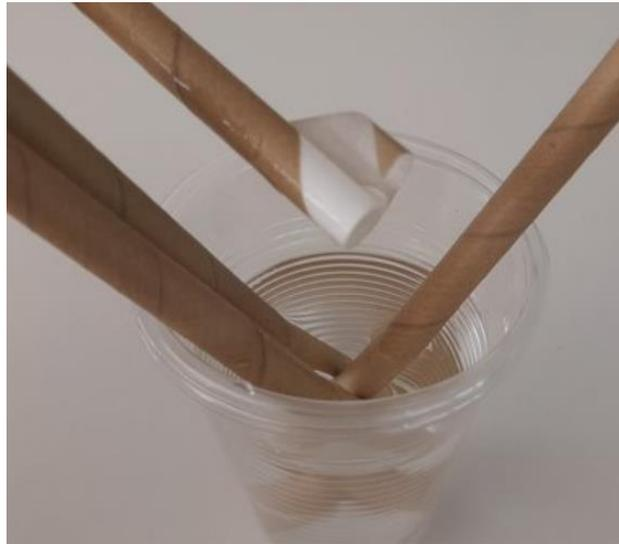
Figure 2: Delamination of paper straw after immersing to water.
