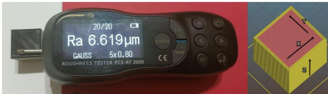
Figure 2: Surface roughness measurement process (left) and determination of measurement axes (right)
