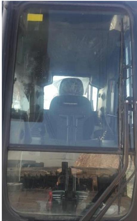
*Figure 14: Test t=60. minute defrosting rate*
