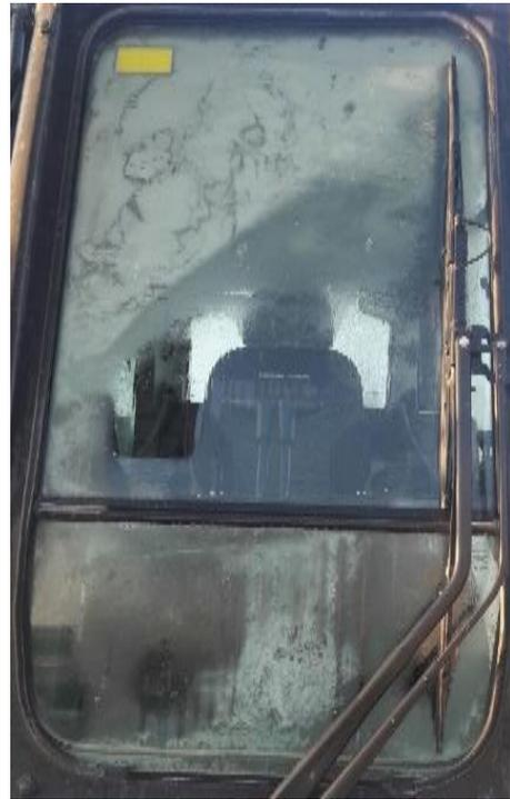
*Figure 11: Test t=15. minute defrosting rate*
