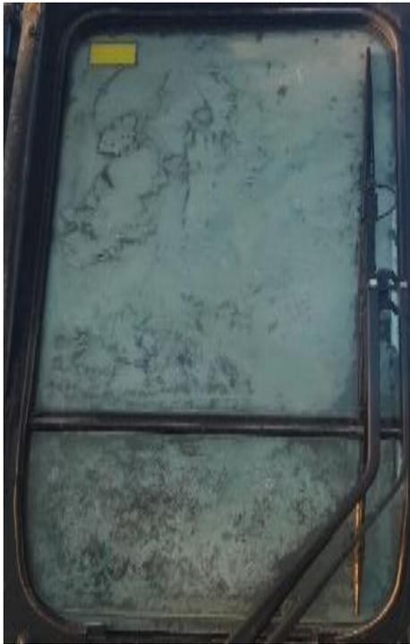
*Figure 10: Test t=0. minute defrosting rate*
