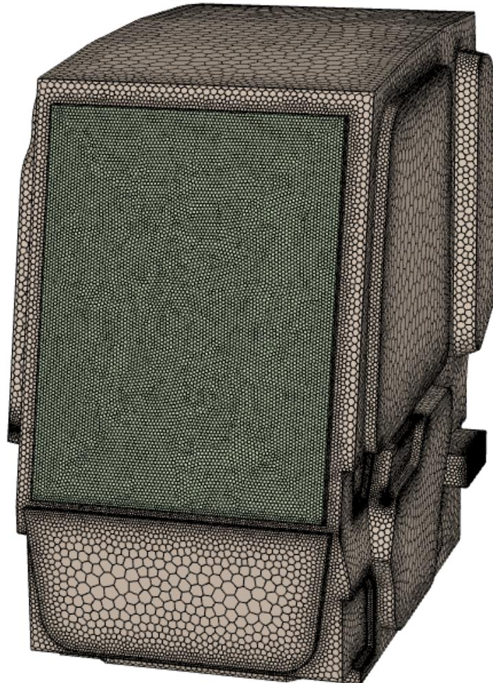
*Figure 3: Cabin mesh structure*
