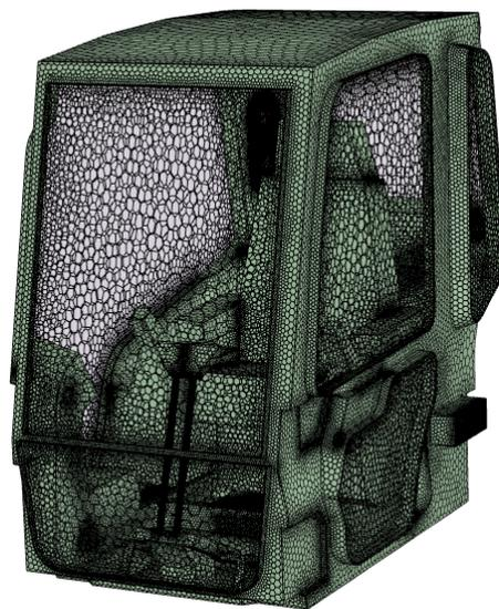
*Figure 3: Mesh view of excavator cabinet*
